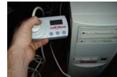
Assessors use meters to determine standby power which can be up to 12% of the total power bill!
